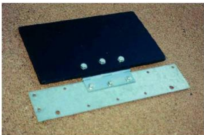
Unpainted, made of Starboard and a cut galvanized framing brace (upside down)
